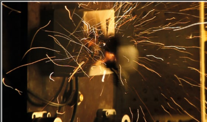
△ An image taken during the testing, showing one of the plugs exploding away from the socket outlet as a result of the catastrophic failure of the fuse.
